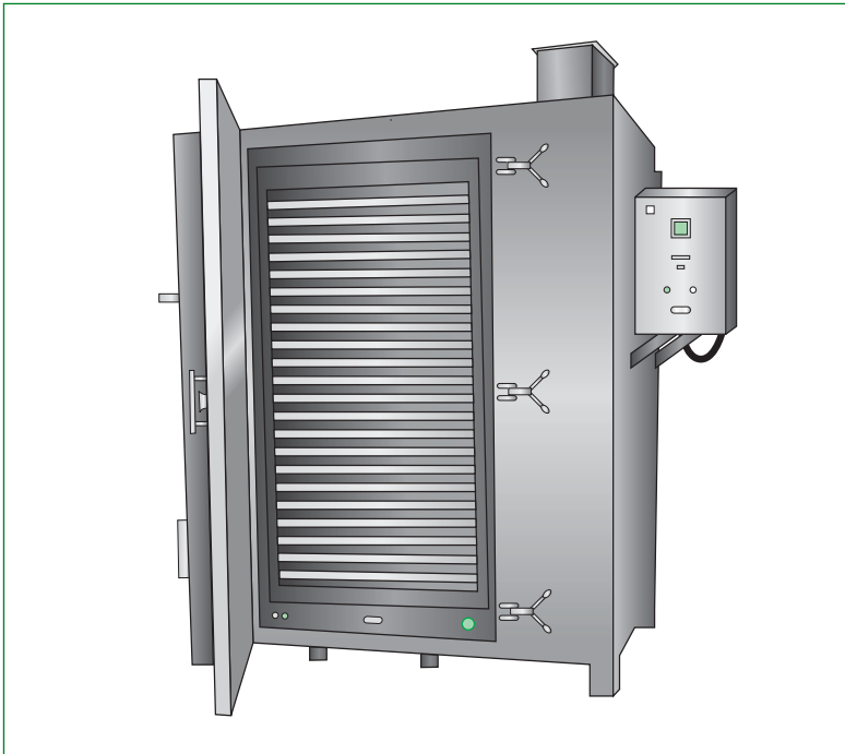
Figure 9.9 An industrial tray drier. (With permission from http://www.chitramachineries.com/products/trayDryer.jpg .)
