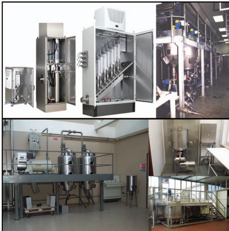
Figure 3.7 Industrial scale ultrasonic devices: (A) probe; (B) bath systems.
