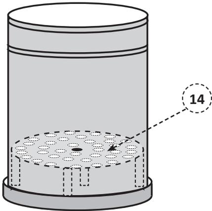
(16) Put No. 10 into a big hole of 2cm diameter when its tongues touch the lower of No.11
