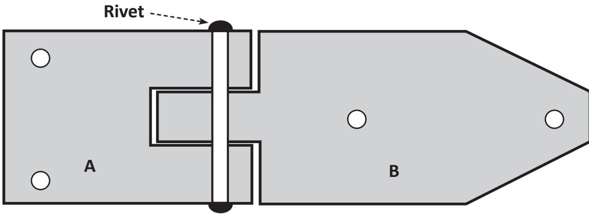
(9) Fix the part of No. 4 to part of No. 7 with a hinge above.
