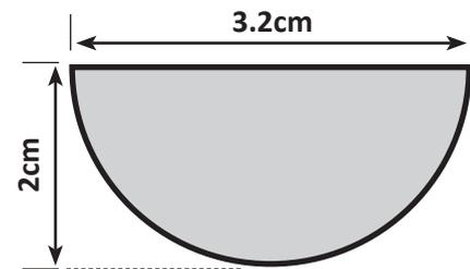
**Note:** All shapes **MUST** be rebated at both ends to stop slide off from the hive.
