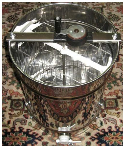
**Fig. 59: A sketch and picture of a honey centrifuge extractor**
