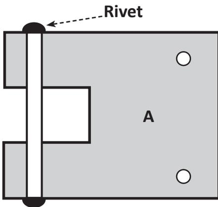
(iii) Put holes as the size of rivets.
