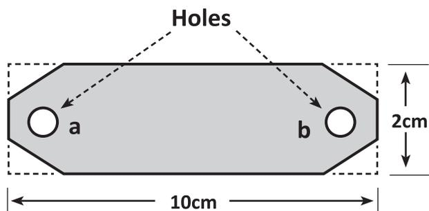
**Fig 46: Measurements and making of a bee smoker:**
