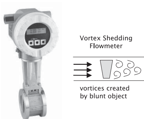
Figure 17.43 Typical Vortex Shedding Flowmeter.
