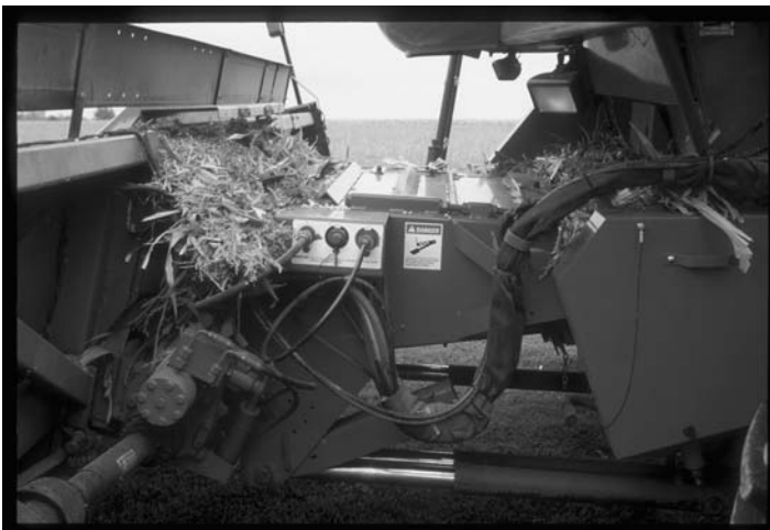
Figure 5.4 Feederhouse connecting head to combine threshing area.
