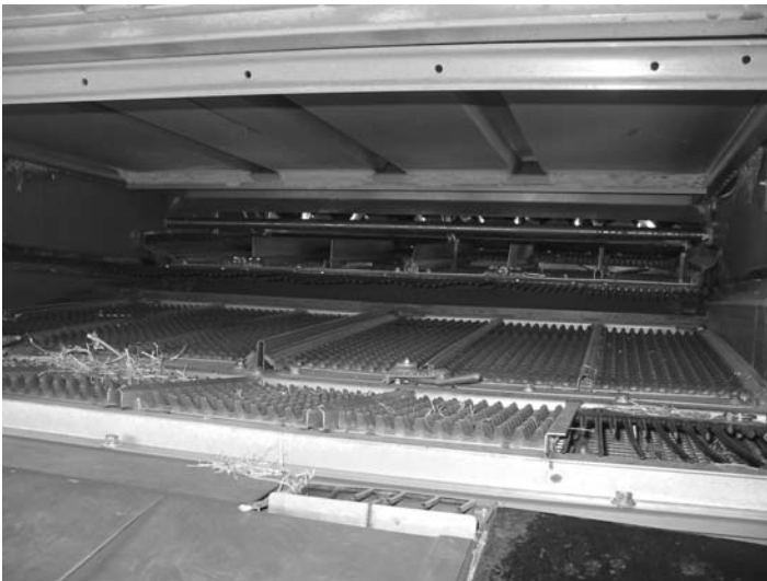
Figure 5.10 Top sieve (chaffer) in cleaning shoe as viewed from rear of combine.
