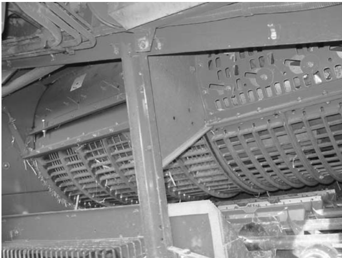
Figure 5.8 Concave around rotor with clean grain augers underneath.
