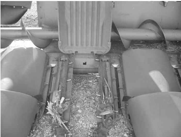
Figure 5.3 Gathering chains and stripper plates over stalk rolls (middle snout is raised).
