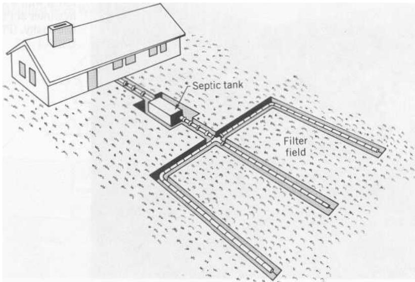
surface. Soils with percolation rates greater than 25 centimeters (10 in.) per hour are unsuited for filter fields because rapid movement of effluent might pollute groundwater.
