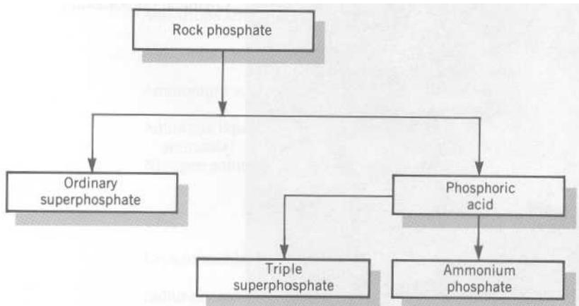
**FIGURE 14.5** Routes for the manufacture of phosphorus materials.
