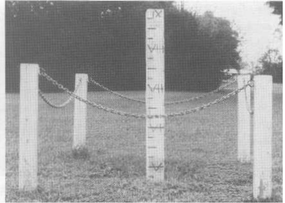
**FIGURE 18.11** In 1924 the bottom of this 9-foot concrete post was placed on the underlying limestone at Belle Glade, Florida, and the top of the post was at ground level. This photograph, which was taken in 1972, shows that subsidence of the organic soil (Histosol) has been about 1 inch per year.
