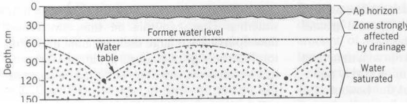
**FIGURE 6.8** The effect of drainage lines in lowering the water table. The benefit of drainage is first evident directly over the drainage lines, and it gradually spreads to the soil area between them.
