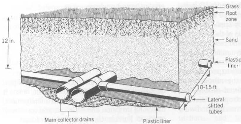
**FIGURE 6.20** Diagram of layout for prescription athletic turf, PAT. The drainage lines remove excess water in wet season and are used for subirrigation in dry seasons. Sensors monitor water and salinity. (Data provided by Prescription Athletic Turf, Inc.)
