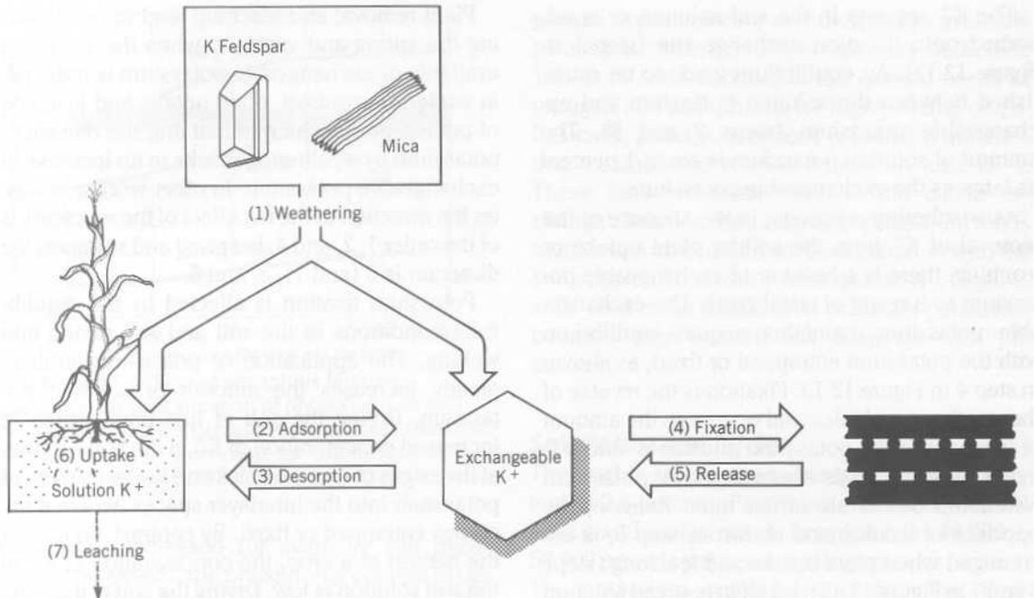
FIGURE 12.13 Major processes in the soil potassium cycle.
